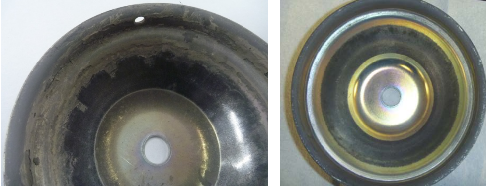
Before and after cleaning cap from left to right respectively
