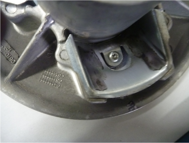
The sliding flange ramps once cleaned
