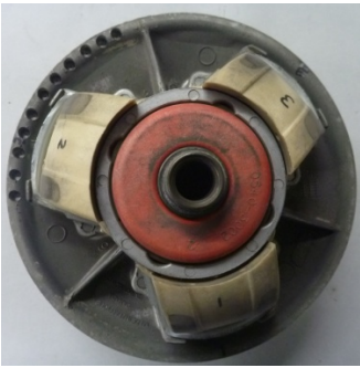
Pulley with the cap are removed
