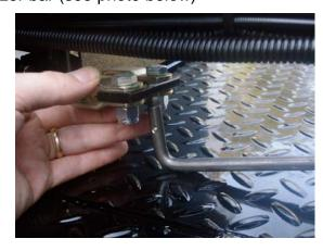
5. Drill a 5/16" hole in the cable bracket on the frame directly between the two brake cables. (Some vehicles may already have this hole.)
