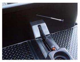
3. Remove the access panel under the parking brake handle then remove the console (cup holders).
