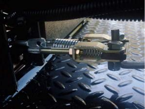
7. At the pedal assembly remove the brake rod clevis bolt (1) (there is no clevis bolt on 4x4 models) and remove the pedal return stop bolt (2). Screw the nut shown below on #2 all the way up to the unthreaded portion of the bolt (2). Using the pedal return stop bolt (2), fasten the brake switch bracket to the floor.
